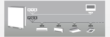
For easier installation and setup, communication wiring can be shared by multiple indoor and outdoor units. \*For Heat Pump systems only
